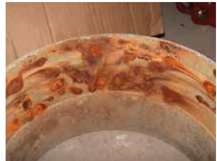
Fig.: Corrosion of pipes
