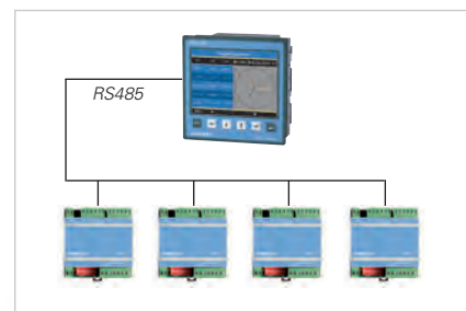
Fig.: Connection of the I/O field bus modules takes place via the RS485 interface of the UMG measurement device
